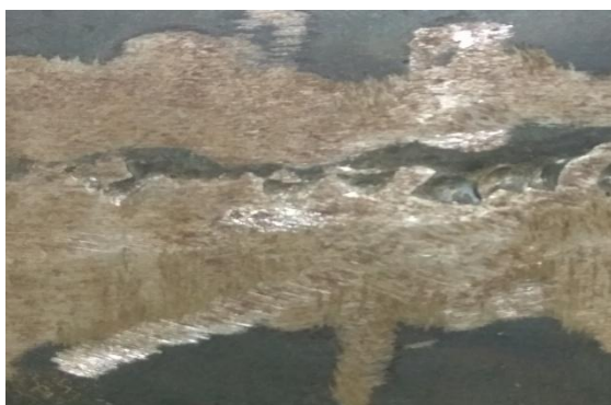
Fig.3 TIG welded steel sheet (Hot & Cold Rolled together)
